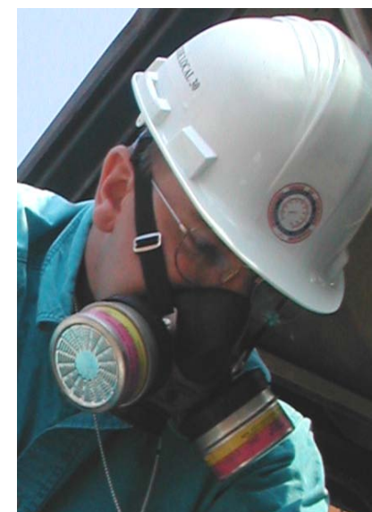
½ face respirator with P-100/OV/AG cartridges
